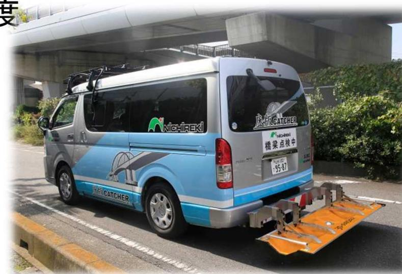
検出幅1.5m ※アンテナ幅1.8m
