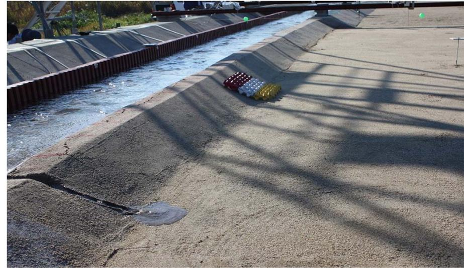
破堤幅 ≒ 40m (t=69min)
