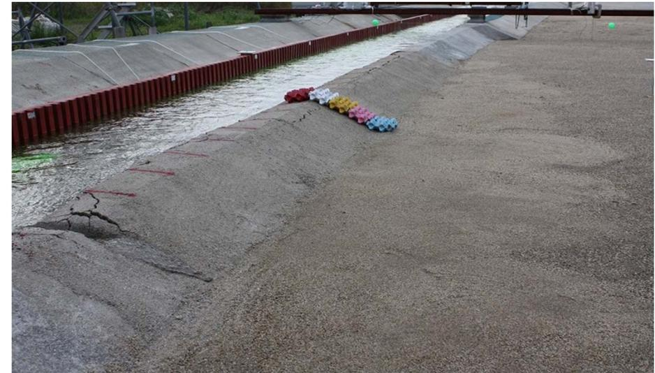
破堤幅 ≒ 40m (t=90.2min)
