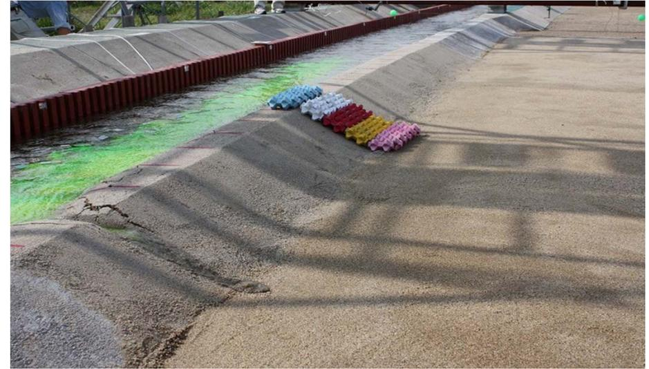
破堤幅  $\approx$  32m (t=35.1min)
